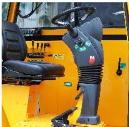
Height and inclination angle adjustable Ecomatic Panel, comfortable for operator.
