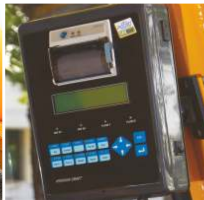
Electronic weighing system cum printer to get quality concrete as per mix design.
