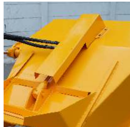
Hydraulic shutter gate to avoid spillage & better loading.
