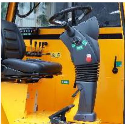
Height and inclination angle adjustable Ecomatric Panel, comfortable for operator.
