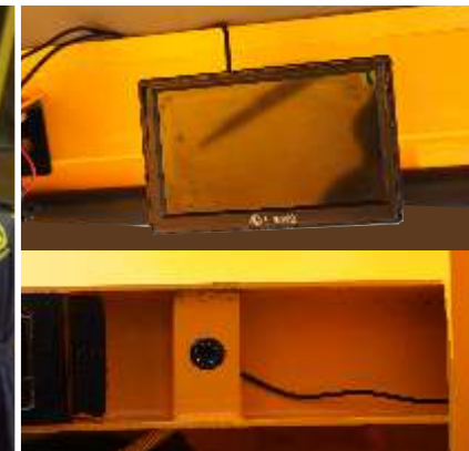
Rear view camera and display for better visibility of the rear portion.
