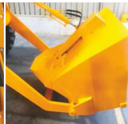
Hydraulic shutter gate to avoid spillage & better loading.
