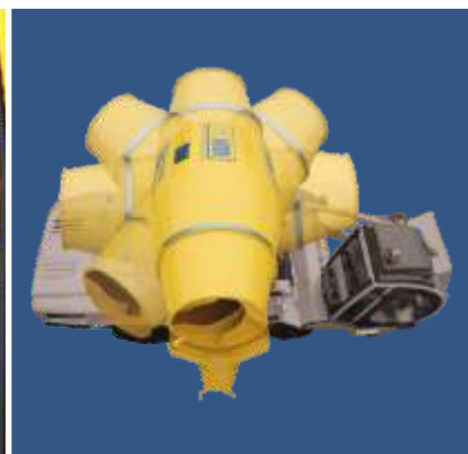
270° Drum Rotation to discharge concrete on all 4 sides of the machine.
