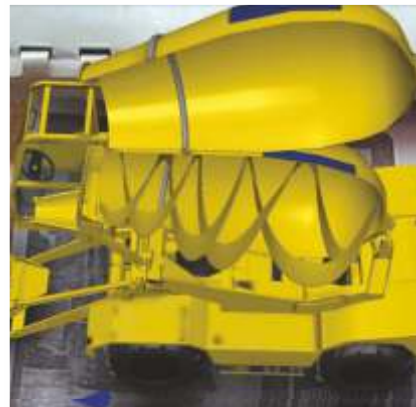
Double helical arrangement with low inclination of drum for better mixing.
